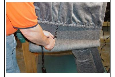
Remove the staples, immediately around the hand wand cord, that attach the magazine pocket to the bottom of the frame.
