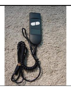
The Okin® hand wand is our low voltage hand wand and is found on most Med-Lift® lift chairs manufactured from 2002 to present.
